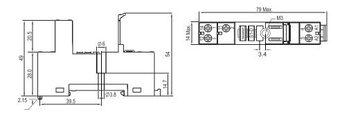
14mm width of the S1D DIN Rail Mountable Socket allows to mount 68 sockets on a Standard 35 mm Din Rail with a length of 1 meter / 1000 mm length (with a provision
